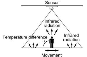
This sensor detects changes in infrared radiation that occur when a person (or object) whose temperature differs from the environment moves.
