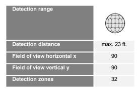
A installation height of 8 ft. results in a detection area of approx. 16 x 16 ft., divided into 32 measuring zones.
